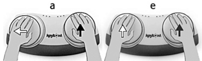
Figure 2: Two inputs, one from each hand, are required to type a character.
